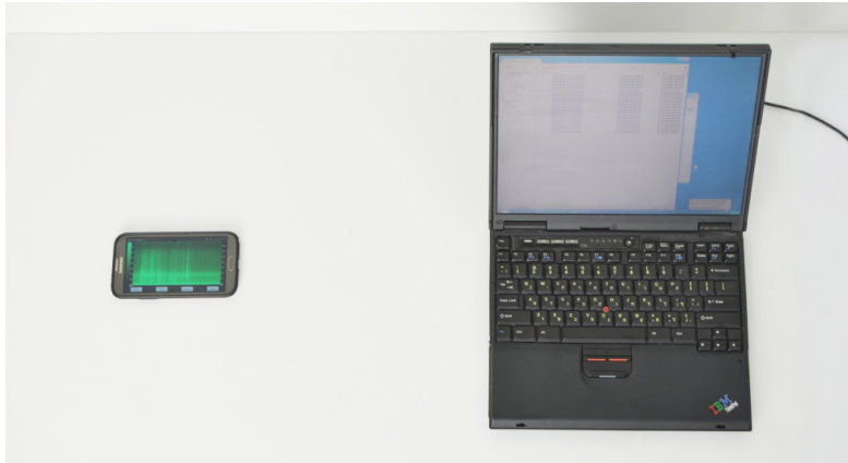
Figure 4: Physical setup of a key recovery attack. A mobile phone (Samsung Note II) is placed 30 cm from a target laptop. The phone’s internal microphone points towards the laptop’s fan vents. Full key extraction is possible in this configuration and distance (see Section 5.4).
